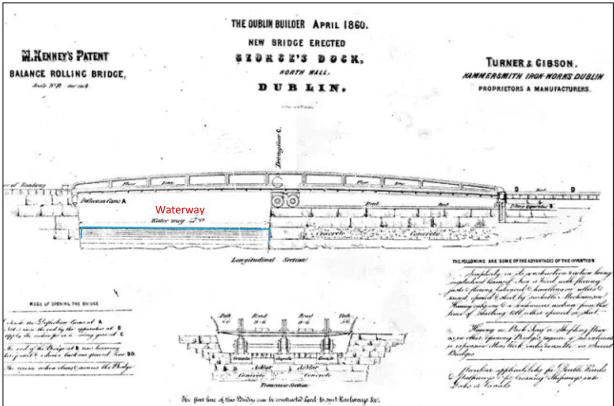
Fig 6.3 Elevation (looking north) and section of drawbridge over entrance to Dock. (*Dublin Builder*, 1860)
