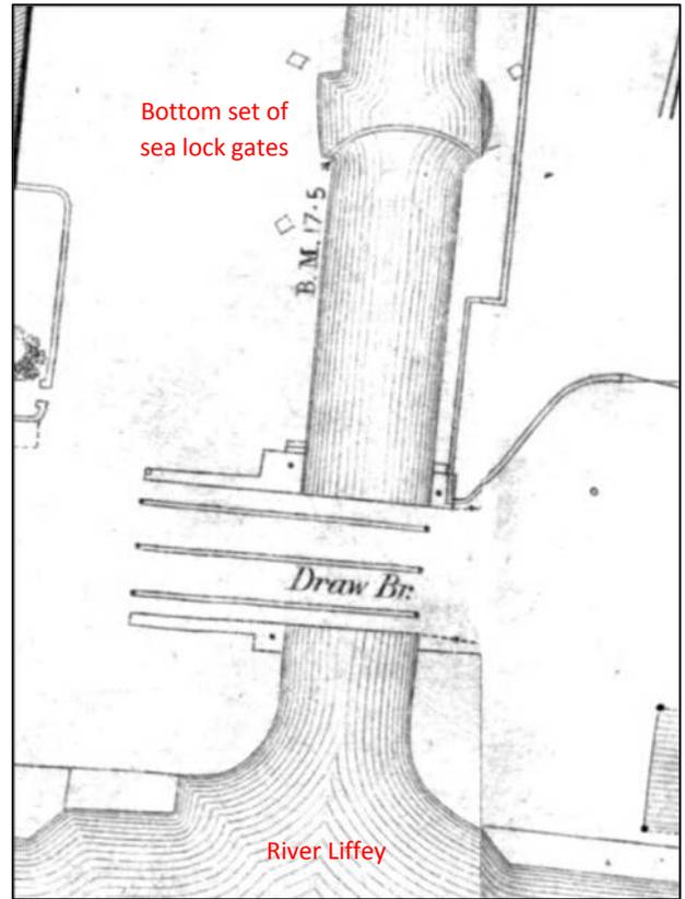
Fig 3.3 1864 map showing the Royal Canal Dock and new moveable bridge at its entrance from the Liffey. The bridge moved west when being opened (*OS 1:1056 map, Dublin City sheets 15 and 16*).
