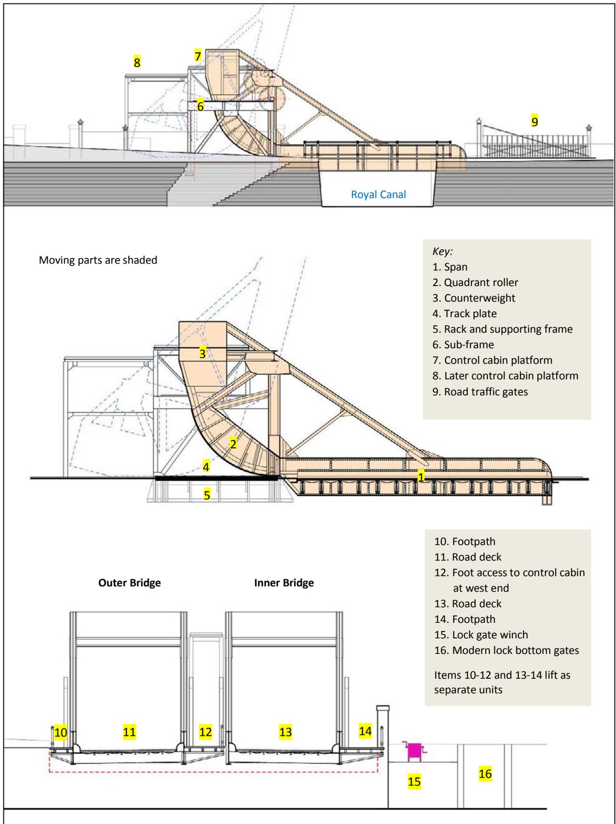
Fig 4.2 *Top*: Elevation of Outer Bridge, from south. *Middle*: Longitudinal section. *Bottom*: Cross-section, from east.
