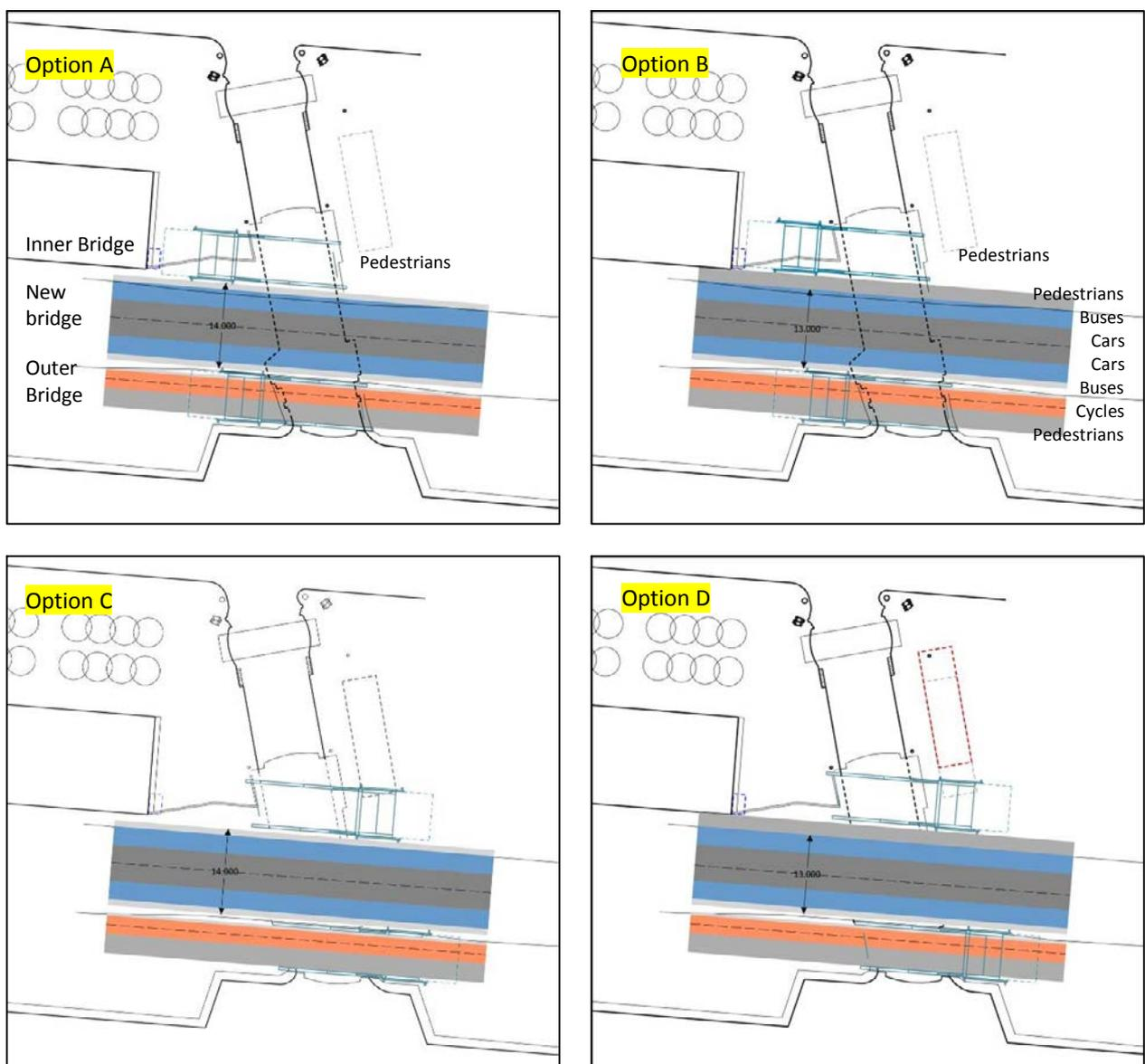
Fig 8.2 Options for repositioning Scherzer bridges.
