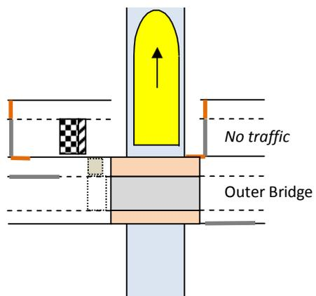
4. Outer Bridge is closed once boat passes under. All road traffic is rerouted across Outer Bridge.
