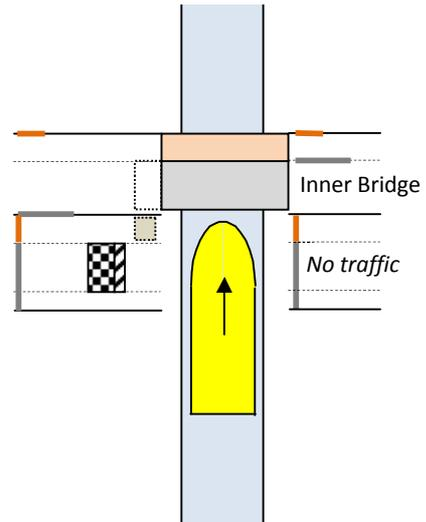
2. Outer Bridge is raised to let boat pass under. All road traffic is rerouted across Inner Bridge.
