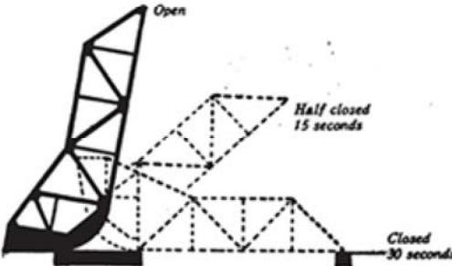
**Scherzer ROLLING Lift Bridges are used *all over the world* because they use the only principle for moving a bridge that anyone would consider for moving any kind of land traffic. They ROLL (or rock) a short distance on *part* of a wheel, just as all land traffic rolls all distances on *whole* wheels.**
