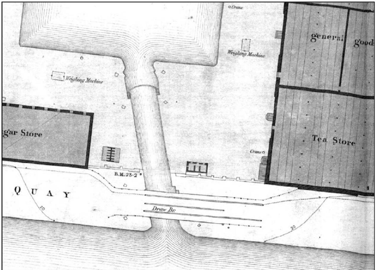
Fig 6.4 1864 map showing the new rolling drawbridge at the entrance to George's Dock. The entire bridge moved eastwards when being opened (*OS 1:1056 map, Dublin City sheet 15*).
