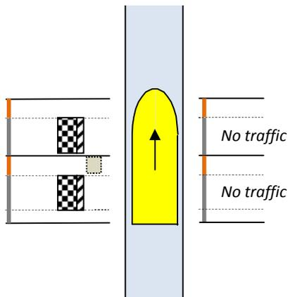
3. Inner Bridge now raised to let boat pass under. Outer Bridge remains raised so both bridges are now closed to all road traffic.
