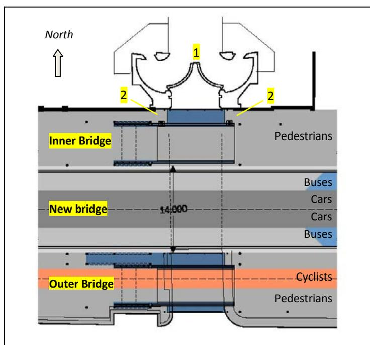
Fig 5.2 Plan of proposed reconfiguration of bridges over Royal Canal. Key: 1 - Sea lock bottom gates (modern); 2 - Winches to operate previous gates (underneath repositioned Inner Bridge).
