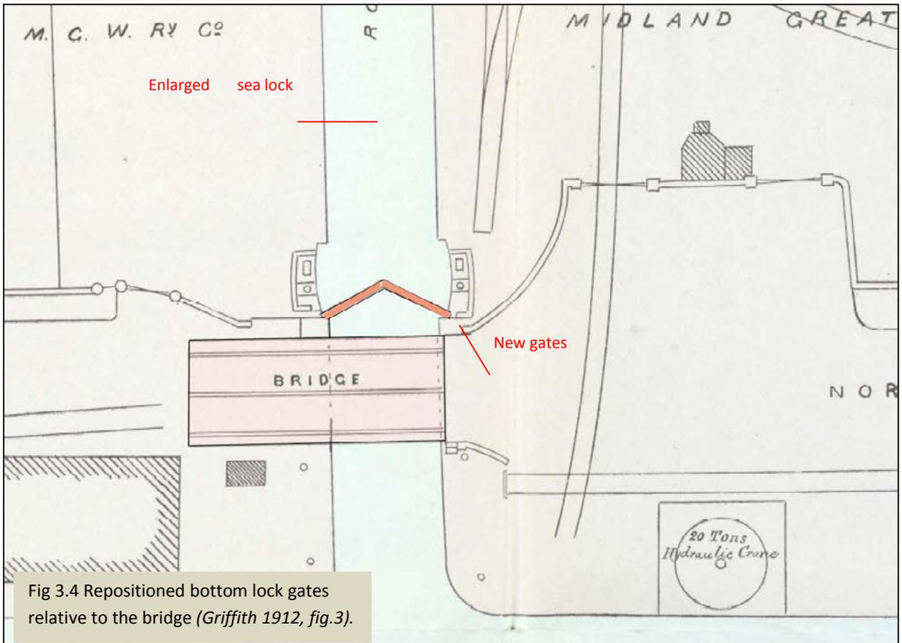
Fig 3.4 Repositioned bottom lock gates relative to the bridge (*Griffith 1912, fig.3*).
