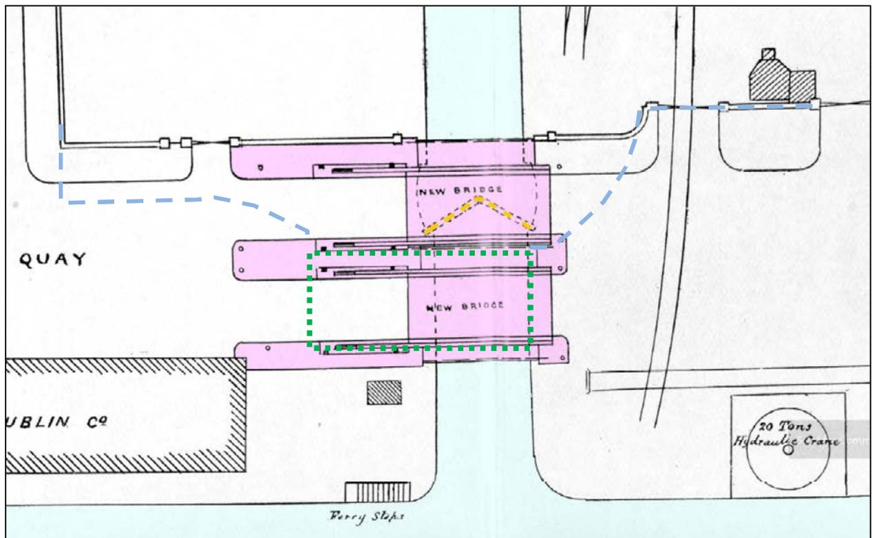
Fig 3.7 John Griffith's Scherzer bridges. The outline of the replaced rolling drawbridge is shown in green. The previous wall along the north side of the road (shown as a dashed blue line) was moved back to accommodate the new inner bridge, under which was the bottom pair of sea lock gates (Griffith 1912, fig.5).
